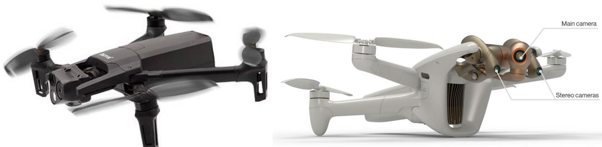
Figure 3: Image of Parrot ANAFI USA (left). This is drone used for most of the shown analyses. On the right is the Parrot ANAFI AI. Images taken from https://www.parrot.com/en/drones/anafi
